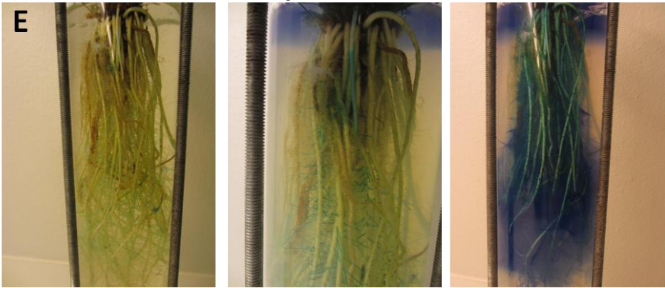
Figure 4-23: Pictures of ROL by plant roots, at 0 h, 2 h and 24 h since the introduction in the agar solution. A: Phragmites australis ; B: Juncus effusus ; C: Cyperus laevigatus ; D: Typha latifolia ; E: Iris pseudacorus
