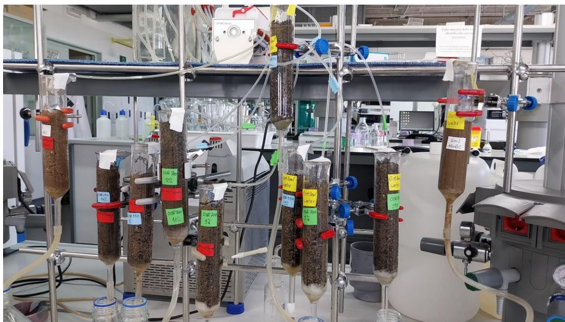
Figure 2. 2. Schematic Representation of the vertical biofilter (VF Soil Filter)
