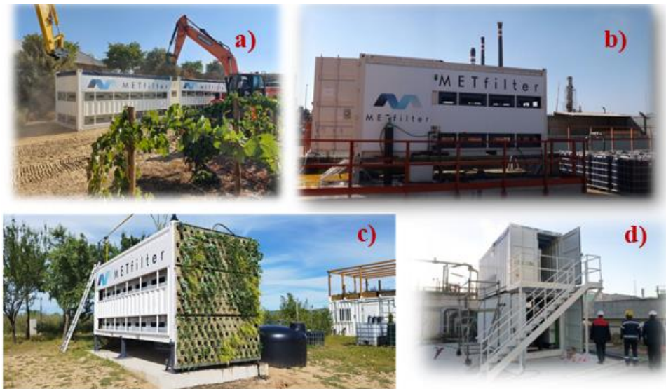
Figure 1. 13. Modular METfilter units for treating wastewater from a) winery, b) petrochemistry, c) urban, and c) oil&gas sector
