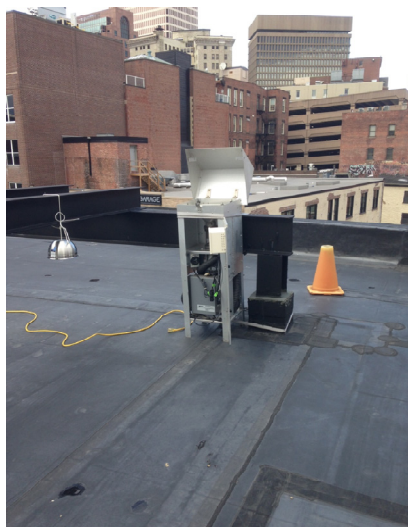
Figure 2.1. A high-volume active air sampler (with opened lid) on a roof in Providence, Rhode Island. On the left, an inverted stainless steel bowl housing a passive air sampling can be seen (Photographed by Rainer Lohmann).
