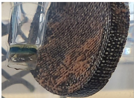
Figure 10. Picture taken of a Geobacter sulfurreducens biofilm on a working electrode acting as an anode in an experimental set-up localized at IMDEA water Institute. Source: author's property.
