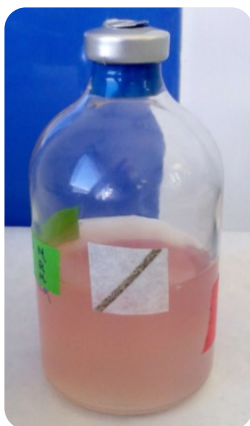
Figure 37. Real photo of culture of Geobacter sulfurreducens in septum-sealed serum bottles.
