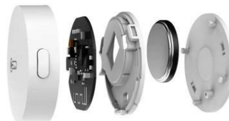
FIGURE 3. ZigBee Xiaomi Mi wireless temperature and humidity sensor [33].
