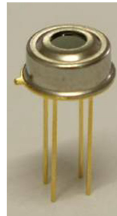
FIGURE 7. MLX90614 contactless temperature sensor [37].
