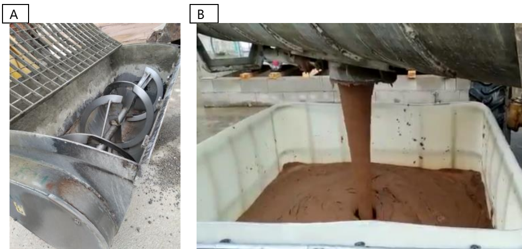
Figure 4.1: Images of A) worm screw homogenizer and B) sediment distribution
