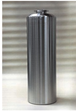
Figure 4.2-9. Stainless steel container for vitrified HLW.
