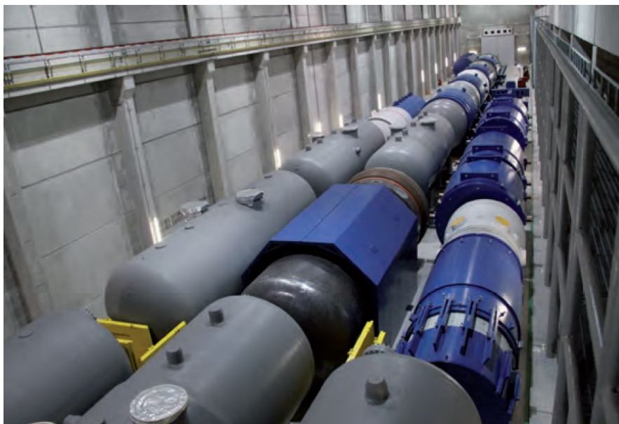
Figure 4.1-1. Decay storage of large components in the storage facility Zwischenlager Nord (Germany)
