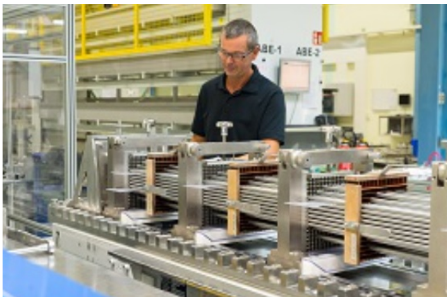
Figure 3.3.4-3. Workbench for assembling fuel assemblies in the Lingen fuel factory of Framatome (Germany)
