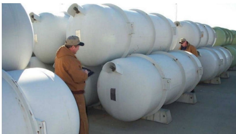
Figure 3.3.3-8. Storage of cylinders with depleted UF_6 at the Portsmouth site
