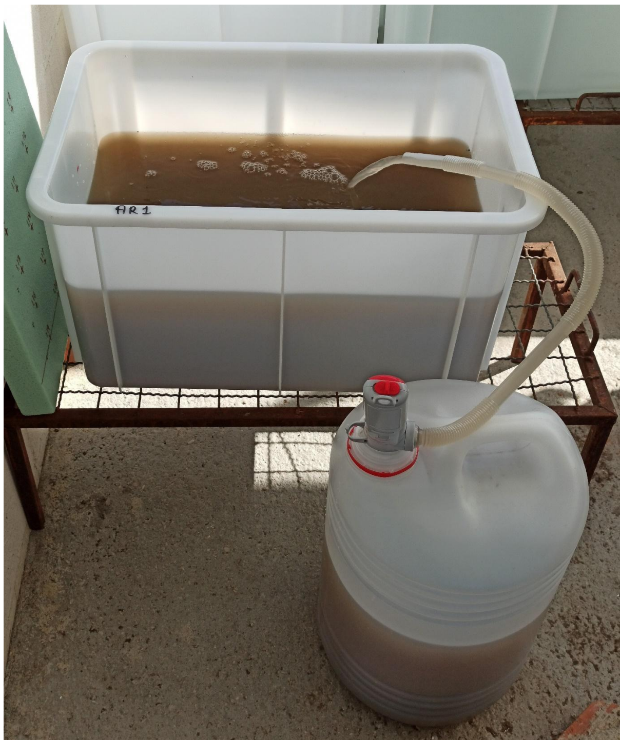
Fig. 3. Buckets being filled with wastewater. The foam slab with one cutting per genotype will be placed floating over the water level.
