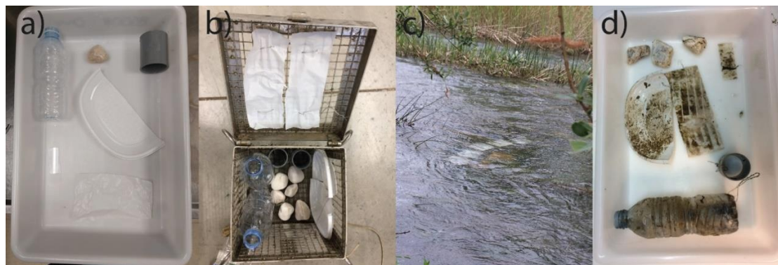
Figure S2. Details of the colonization process: a) Virgin substrates previous to the colonization experiment, b) Distribution of the different substrates in the metal cage, c) Deployment of metal cages with plastics inside the river, d) Condition of the substrates after 1 month of colonization.
