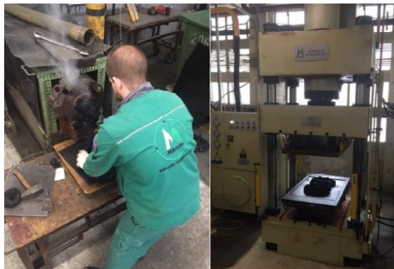
Figure S 3. Hot melt taking out from the extruder and putting into the mould.
