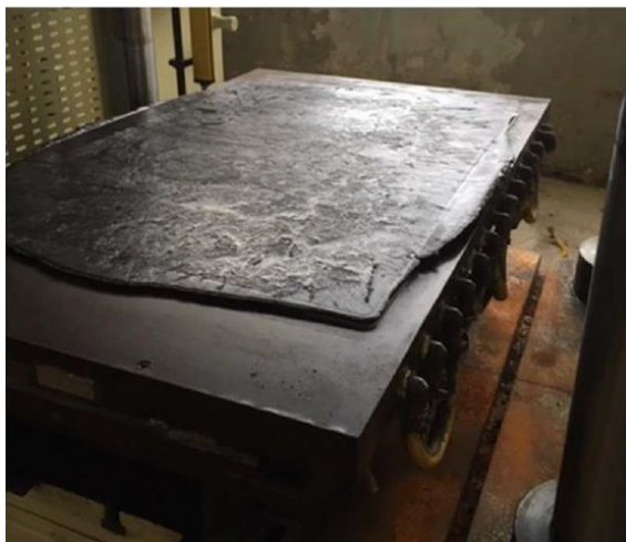
Figure S 4. Flat sheet after moulding and cooling down.
