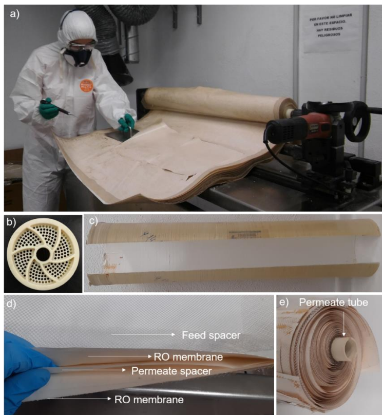
Figure 14. Deconstruction of the EoL RO membrane for its indirect recycling. a) membrane autopsy (taking out membrane coupons) (From [71]), b) end cap, c) fiberglass casing, d) disposition of the feed spacer, RO membrane and permeate spacer in the spiral wound module, e) permeate tube.
