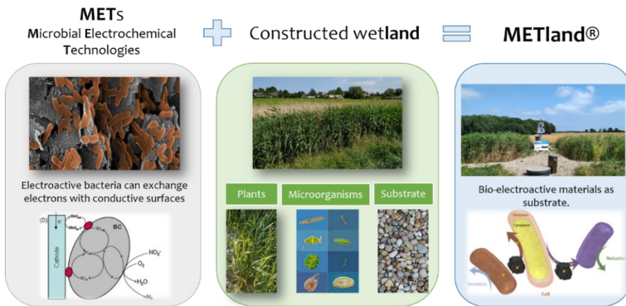
Figure 1.11. METland concept, merging METs and constructed wetlands.
