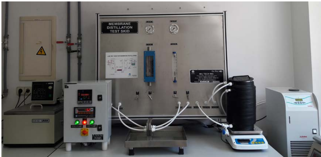
9 Fig. 4. Schematic and real images of the DCMD long-term experimental set-up.
